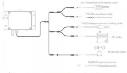
▲ Supports up to 5 probes simultaneously, 1 of each type.
